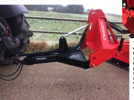
This well thought out product is built in high strength steel and is the only product in the market which has a unique turntable with changeable wear plates.
